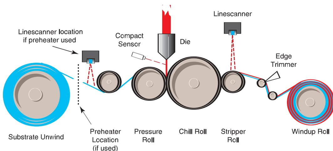
Figure 5: Extrusion Coating Process
