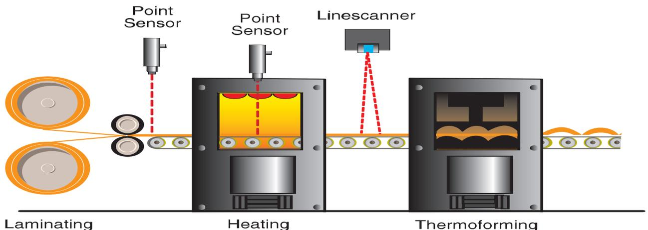
Figure 7: Thermoforming Process
