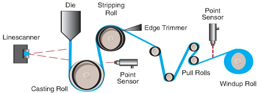
Figure 2: Cast Film Extrusion Process
