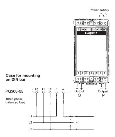
The same connection diagrams for connection via current resp. voltage transformer.
