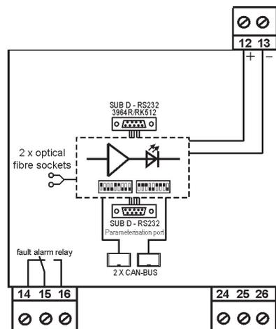
Basic module with additional serial interface
