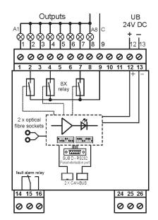
Basic module with 8 output relays
