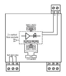
Basic module with additional serial interface
