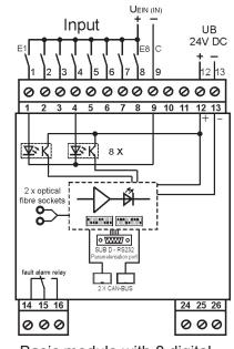
Basic module with 8 digital inputs
