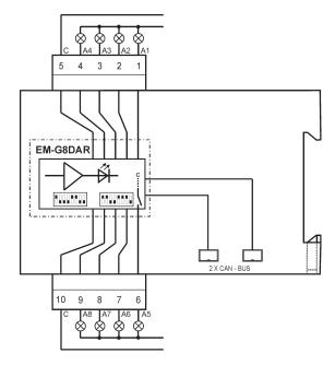
Terminal assignment of the relay module
