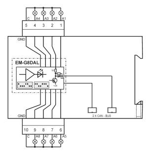
Terminal assignment of the transistor output module
