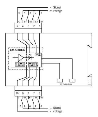
The 8 inputs are realised in 2 groups of 4 inputs with a common root. The 2 inputs groups are potentionally isolated against each other.
