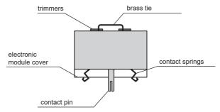
Fig. 15: Side view of the electronic module
