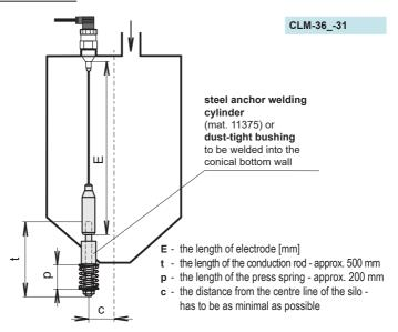
Fig. 7: Installation of rope electrode with anchor
