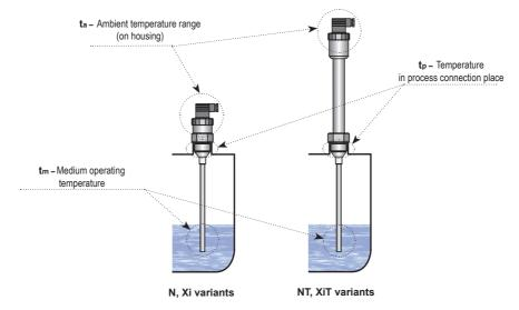
Fig. 17: Points for temperature determination on the level meter
