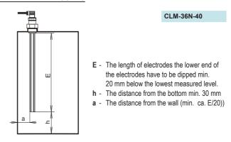
Fig. 8: Installation of level meter with reference electrode
