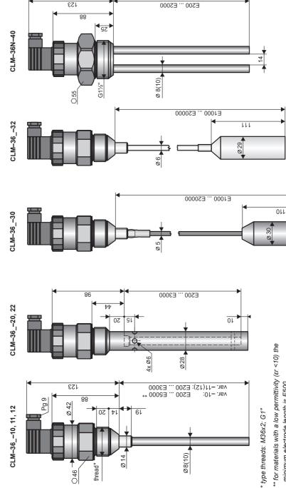
Fig. 1: Dimensional drawings of the capacitive level meters
