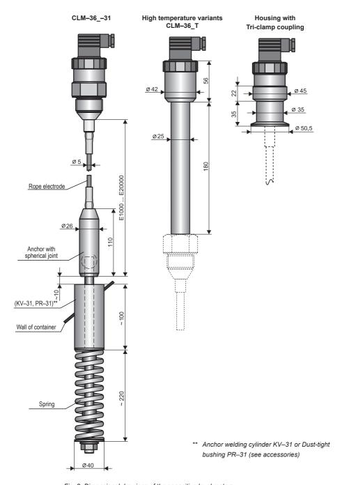
Fig. 2: Dimensional drawings of the capacitive level meters
