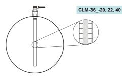
In the tank with straight wall (for example vertical cylinder) and with the sensor placed parallely with the wall capacity change is linear.
