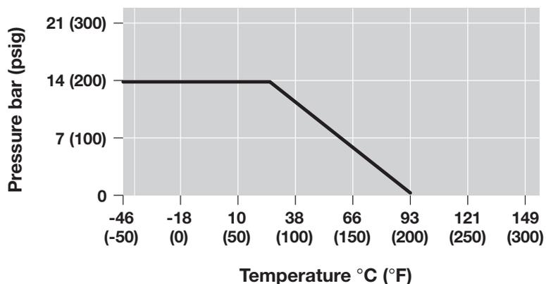
Maximum Pressure ratings for CRN are derated to 130psig (-1 to +9 bar) @70° F (20° C)
