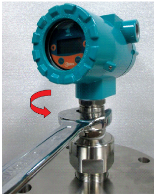
Rotation at Union Joint Max 360° allowable one-time rotation in either direction.
