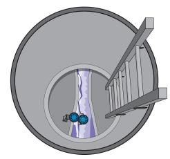
NOTE: For optimal accuracy, mount the transmitter a minimum of 75 cm (30") above the flow element (this is dependent on type and size of the flow element). Consult factory for assistance on this dimension.
