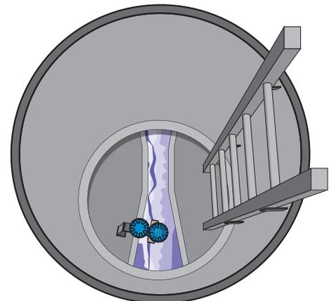
NOTE: For optimal accuracy, mount the transmitter a minimum of 75 cm (30") above the flow element (this is dependent on type and size of the flow element). Consult factory for assistance on this dimension.
