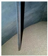
Continuous filling with build-up on probe
