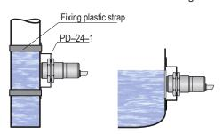
CPS sensor application for level gauges and eye sights
