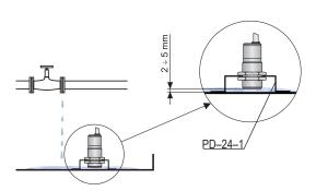
Use of CPS for sensing leakages in an interception tank
