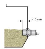
Sensing bulk-solid materials in storage tanks
