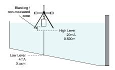
Typical installation - Set 'Low Level' (4mA) to be the distance from the transducer face to the bottom of the tank. High Level should be 0.500m for most accurate and reliable measurement.
