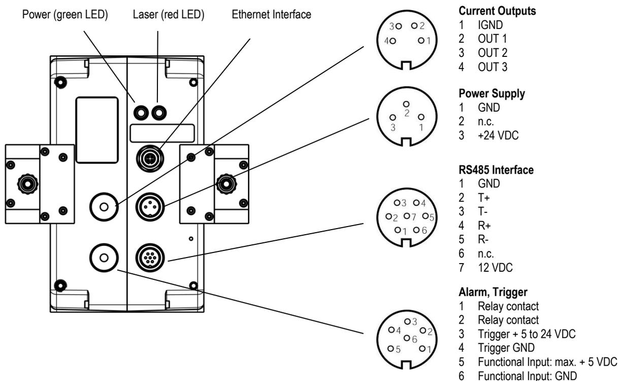
Figure 8: Input and Output Connectors (view on connectors)
