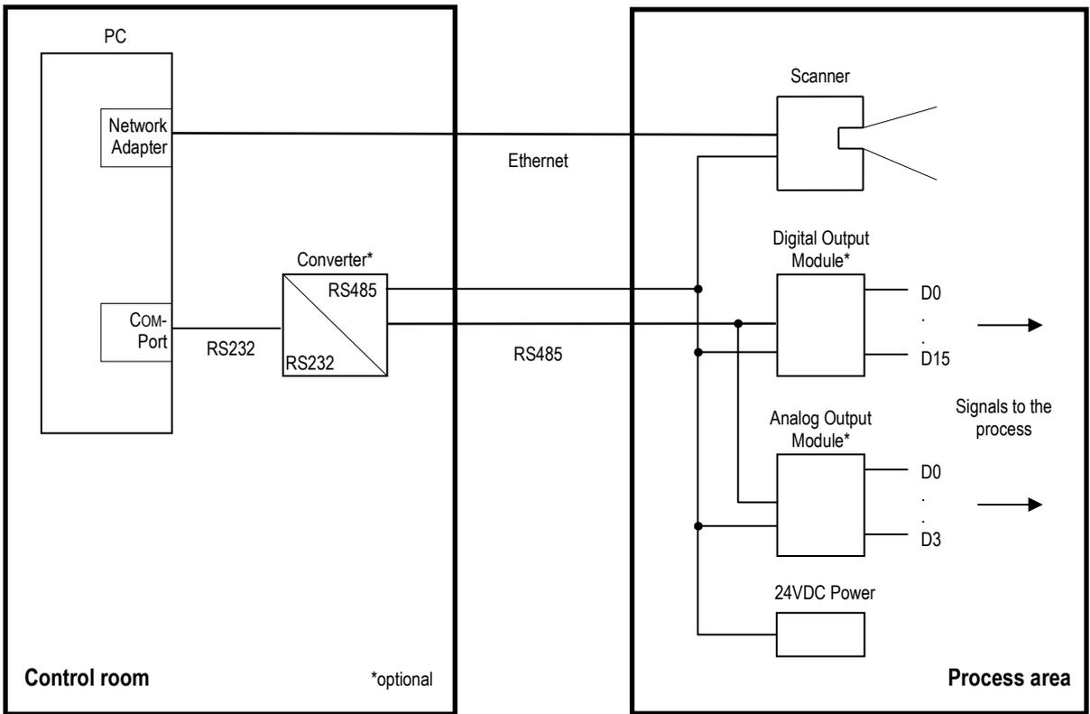
Figure 21: Principal Installation of Serial Output Modules
