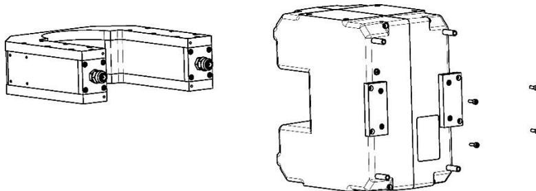
**Figure 33: Removing the air purge collar**
