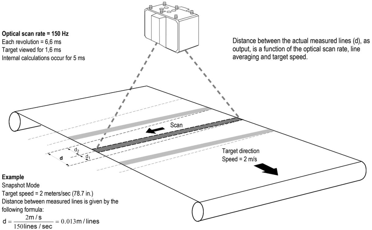
i.e., During 100% mirror rotation, which takes 6,6 ms, target moves  $d = 0.013\text{ m}$  (0.51 in.)
