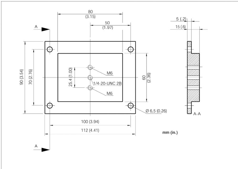
Figure 14: Mounting plate for tripod with 1/4" thread
