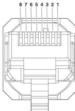
Figure 11: RJ45 Connector
