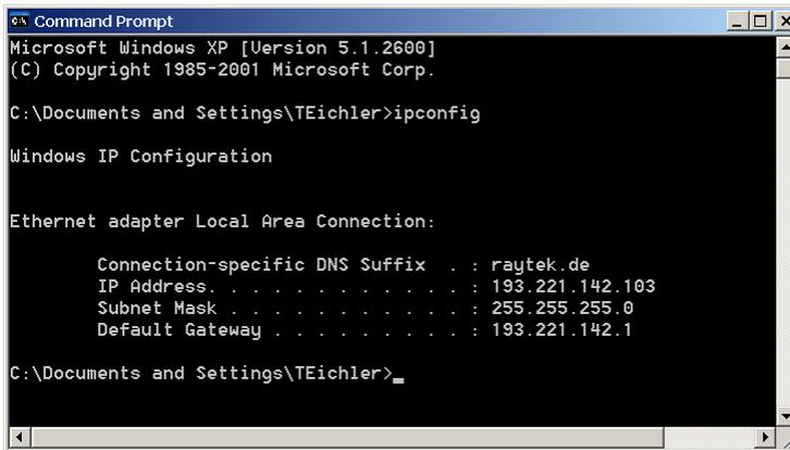
For the example above, the IP address of the PC is 193.221.142.103. The subnet address is 193.221.142, the host address is 103. The scanner's subnet address must be 193.221.142 as well. The host address of the scanner must be in the range from 1 to 254 with the exception of 103 which is already used for the PC.
