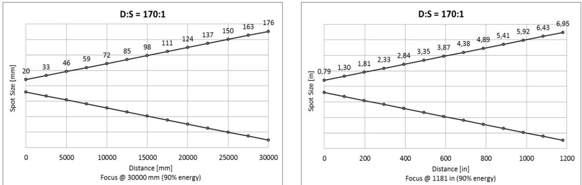
Figure 4: Optical Diagrams Far Focus
