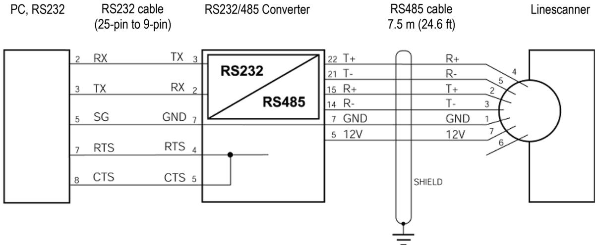
Figure 18: RS232/485 interface between linescanner and PC
