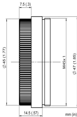
Figure 43: Dimensions for Protective Window
