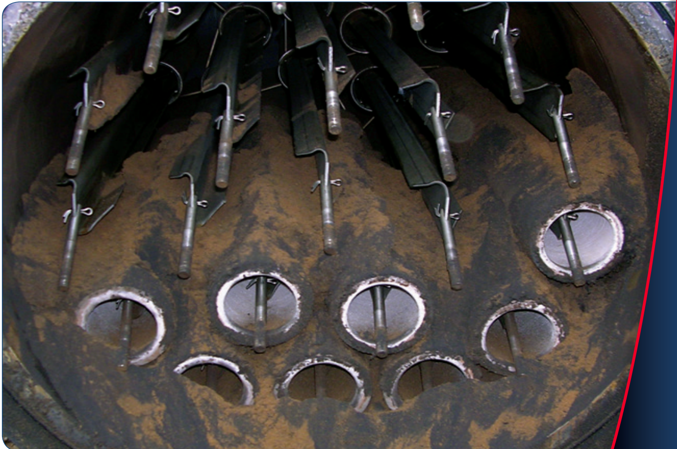
Model 75H Filter-Separator loaded with contaminants
