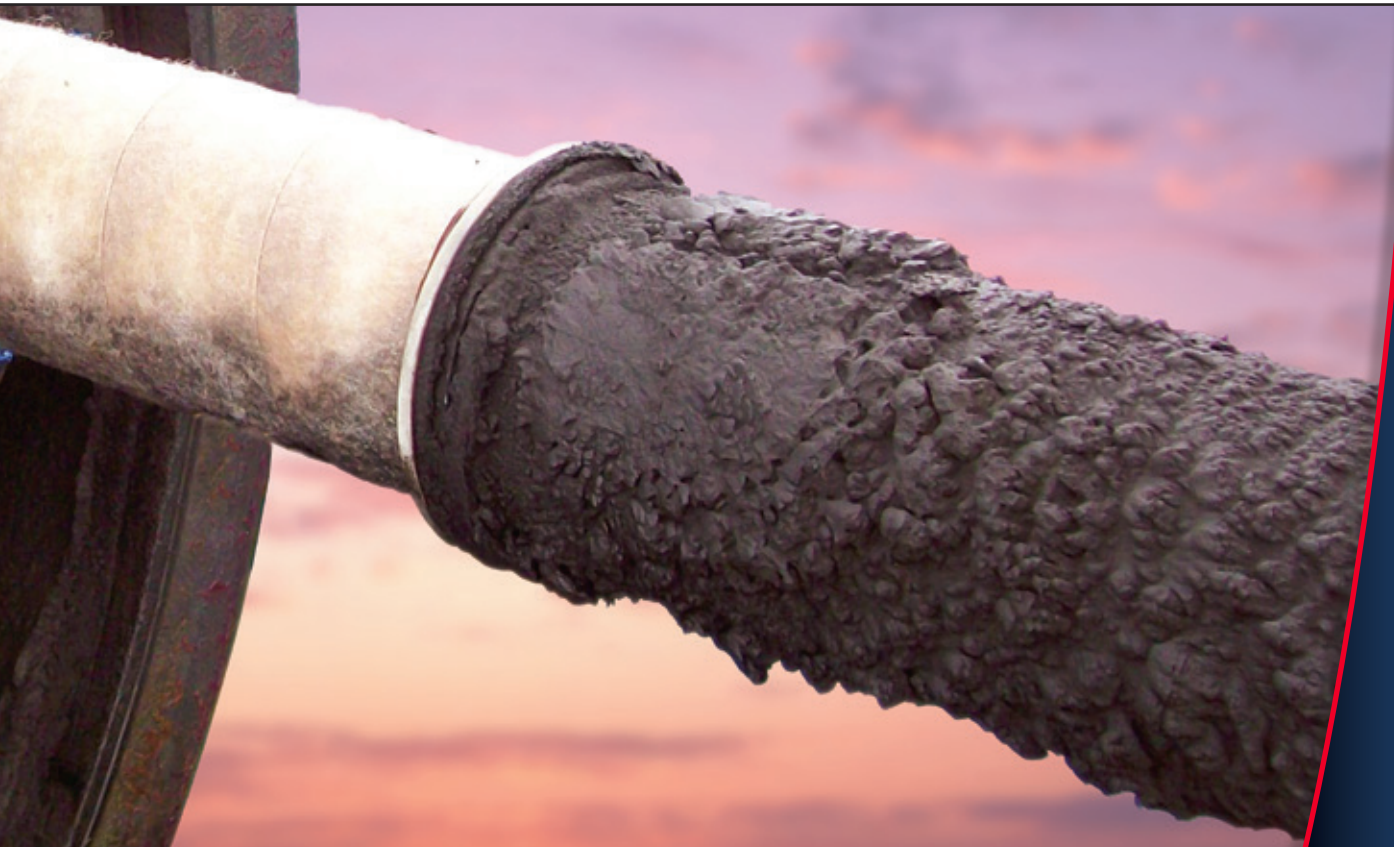
Spent PEACH® Gemini Model PGC cartridges from field
