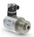
2/2 way valve direct acting pressure range PN 0-400 bar orifice DN 2-8 mm connection thread function valve
