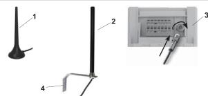
The FME jack of the magnetic base antenna [1] or the optional outdoor antenna [2] is screwed into the FME plug [3] of the module. To guarantee optimal reception, the antenna should be mounted outside meter cabinets, upright on a magnetic surface.
