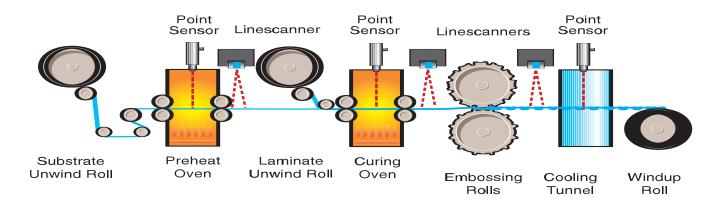
Figure 6: Laminating and Embossing Process
