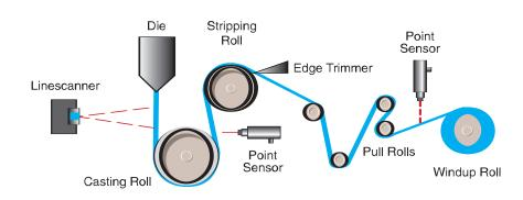
Figure 2: Cast Film Extrusion Process
