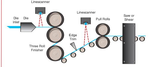
Figure 3: Sheet Extrusion Process
