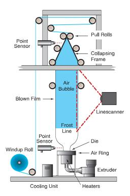
Figure 1: Blown Film Extrusion Process
