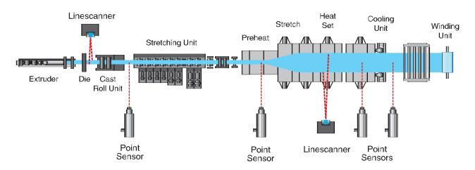
Figure 4: Biaxially-oriented Film Extrusion Process
