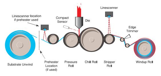
Figure 5: Extrusion Coating Process
