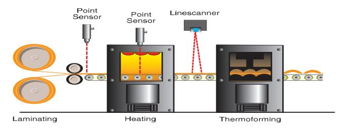
Figure 7: Thermoforming Process
