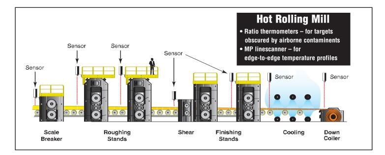
Either way, the stands' rolls must be set to compensate for the temperature change.
