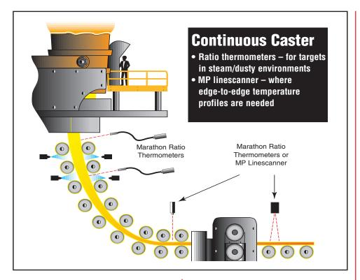
Accurate ongoing temperature measurements are crucial throughout the steelmaking process to produce quality products and enhance process efficiency.
