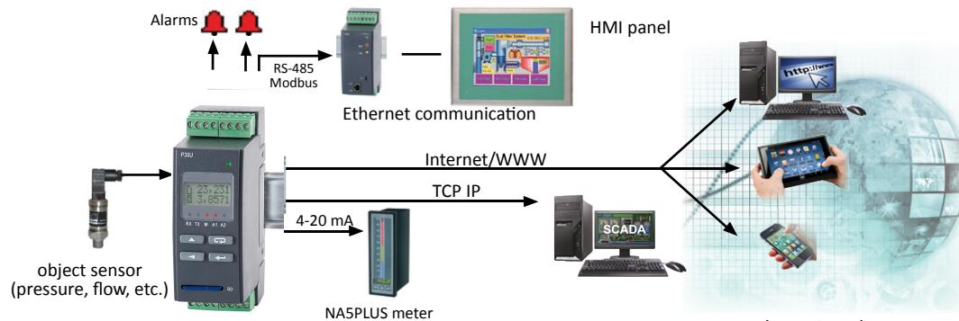
Measurement and signal conversion with its visualization and retransmission.
