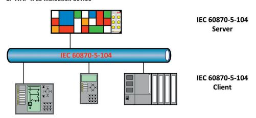
In this application example the WAP-K processes and displays alarms that are retrieved from the IEC interface. Thus, a secondary wiring of the alarms is not necessary.
