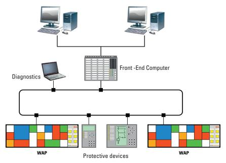
With the optionally available software license IEC 61850 the WAP-K can be integrated into IEC 61850 structures.
