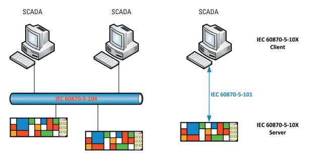
In the application example above, the WAP-K annunciators work as acquisition devices, which processes and displays alarms locally. In addition the alarms are forwarded to the SCADA level through IEC 60870-5-101 or -104.
