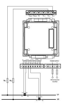
Measurement in single-phase system with or without voltage transformer
