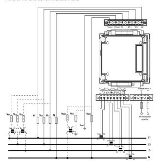
Three-phase measuring with or without voltage transformer and MC3 (250 mA) + .../5 A type transformers for neutral current.
