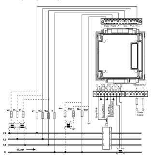
Direct phase-phase measurement with current transformers
