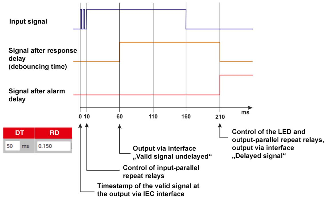
Fig. 5.19: Time diagram with a response delay of 50 ms and a alarm delay of 150 ms
