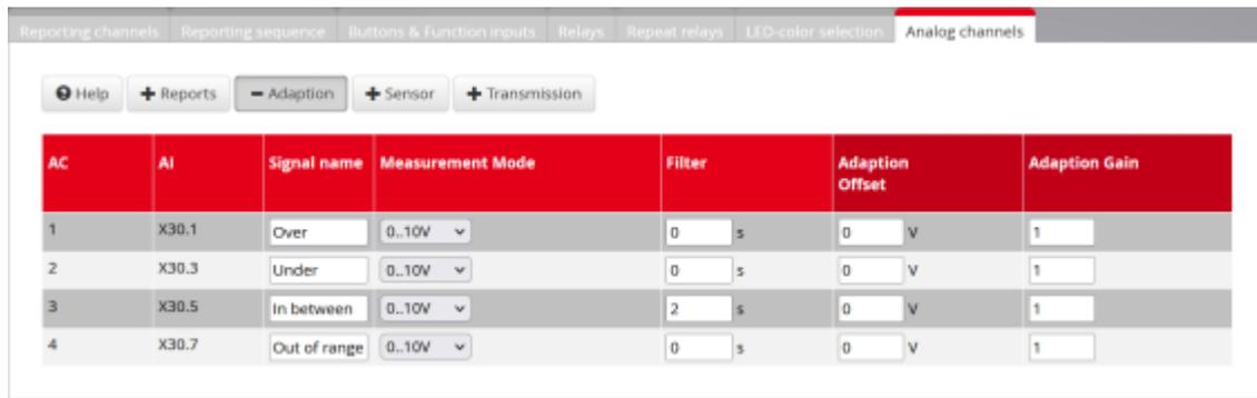
Fig. 5.26: Submenu analog channels - Dialog adaption
