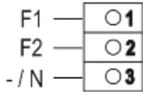
Fig. 3.10: Terminal assignment of the function inputs
