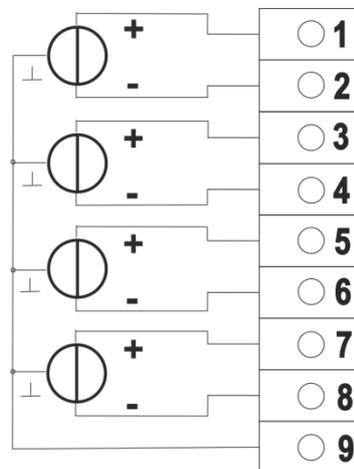
*Fig. 3.17 Sensors with differential output*
