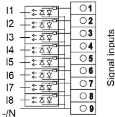
Fig.3.11: Terminal assignment of the signal inputs
