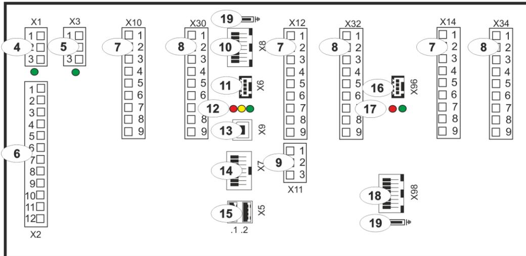
Fig. 3.8: Back view of the USM24
