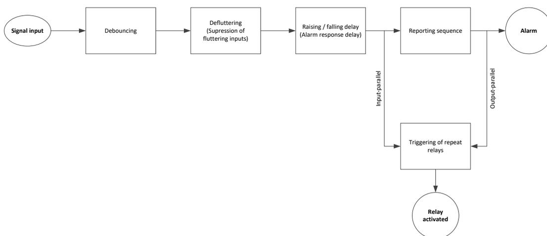
Fig. 5.18 Schematic illustration of the alarm processing in the annunciator
