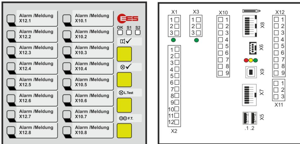
Fig. 3.19: Front and back view of the USM 16 in housing 96 x 96
