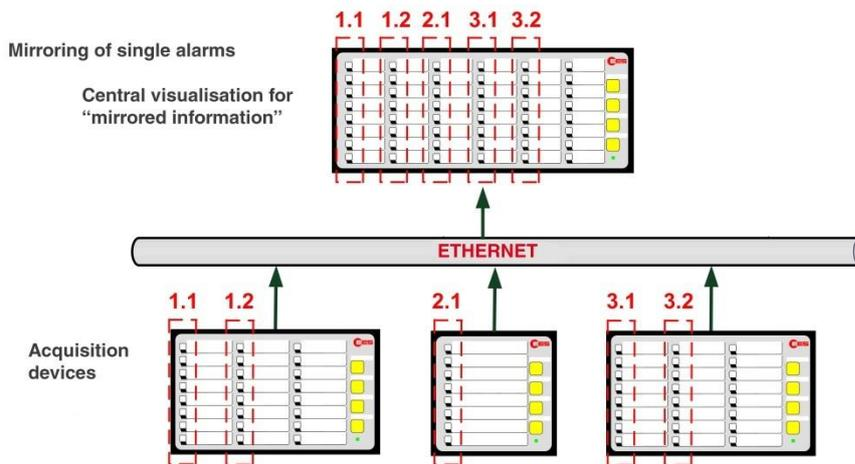
Fig. 3.4: Application example for mirroring
