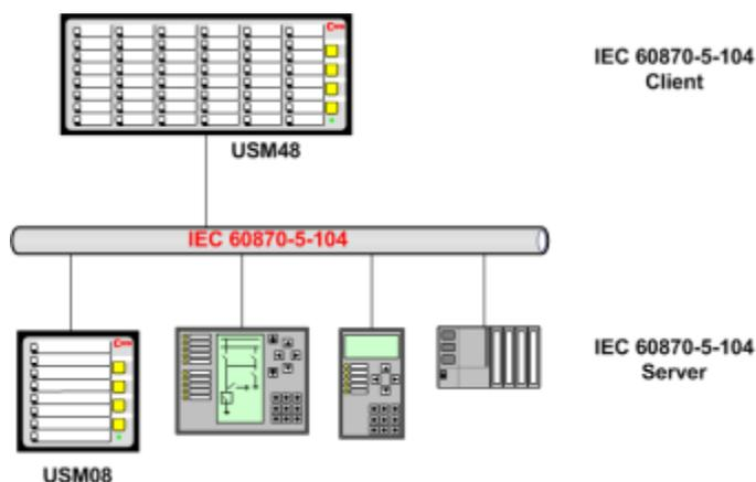
Fig. 3.3: Application example with USM as an output module
