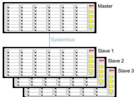
Fig. 5.9: Example of a cascaded annunciator system
