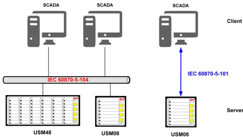
Fig. 3.2: Application example for communication of USM acquisition devices (IEC-Server/Slave) with an IEC-Client/Master.
