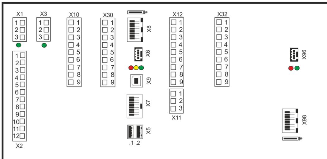
Fig. 3.21: Back view of the USM 16W in wide housing 96 x 192
