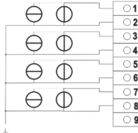
*Fig. 3.15: Sensors with common reference ground (Ground connected to sensor)*
