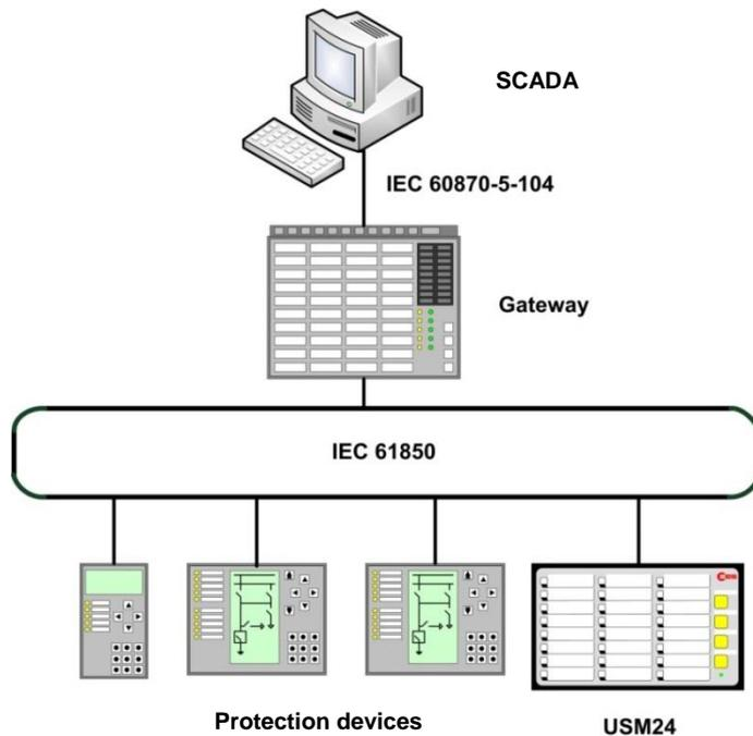
Fig. 3.5: With the optionally available software license IEC 61850 the USM can be integrated into IEC 61850 structures
