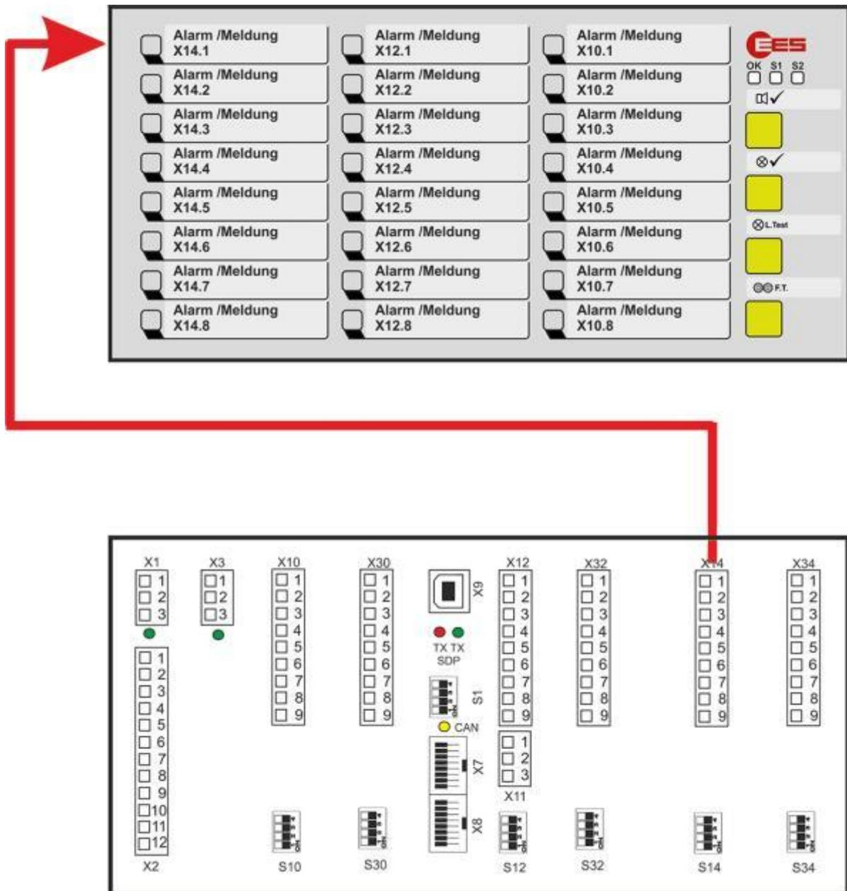
Fig. 3.32: Assignment between alarm input and LED display using the example of a USM 24
