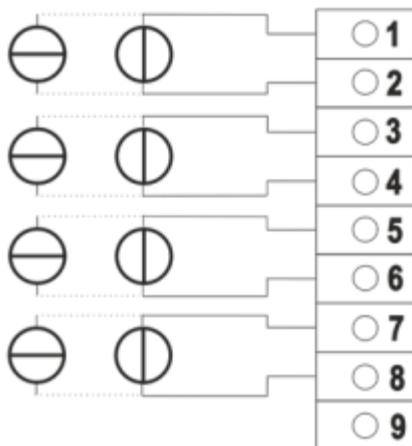
*Fig. 3.16 Sensors with common reference ground (Ground connected to the input terminals)*
