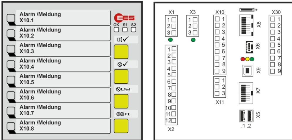
Fig. 3.18: Front and back view of the USM 08
