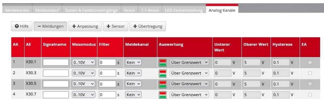
Figure 5.25: Analog channels submenu for a fault annunciator with 2 analog cards with 4 inputs each
