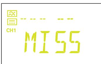
The installation has changed and the device does not find the **WGB**.
