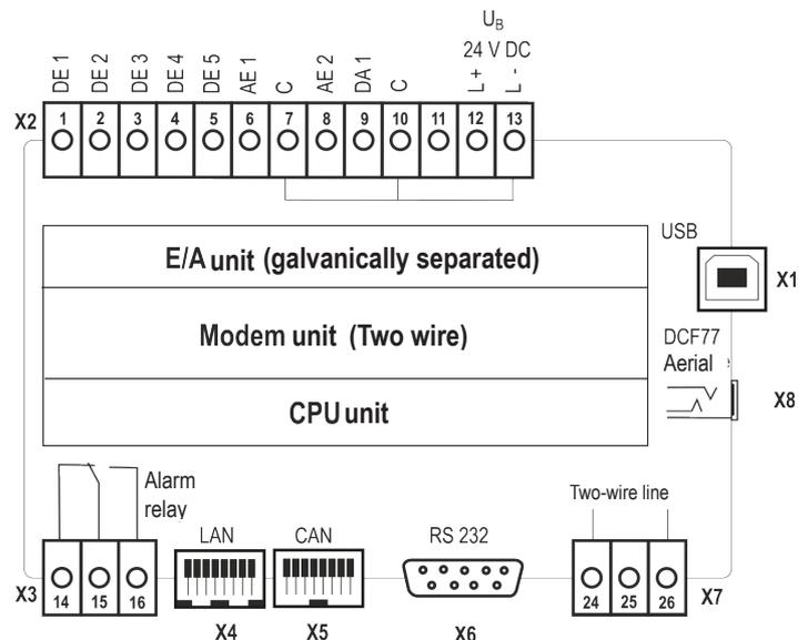
Basic module with 5 DI, 2 AI and 1 transistor output
