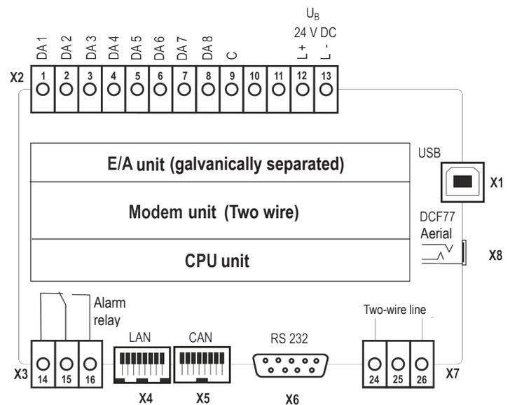
Basic module with 8 output relays
