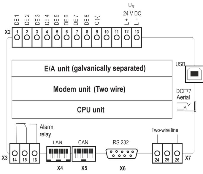
Basic module with 8 digital inputs
